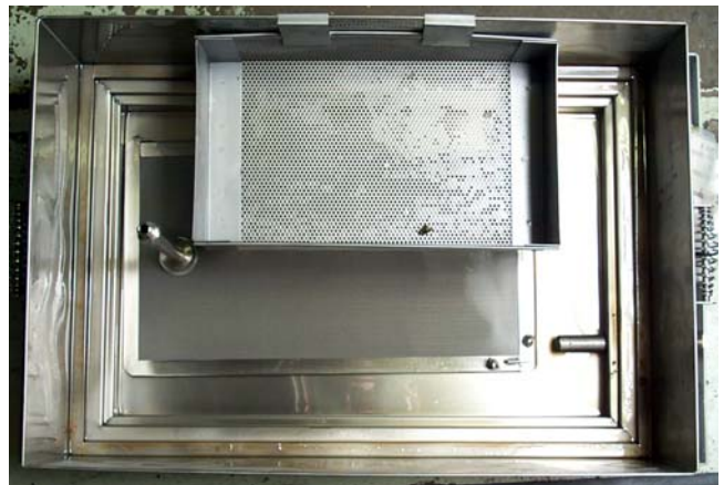
Crumb screen properly placed in filter pan.
